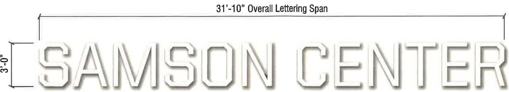
5 FRONT VIEW / SIGN ST-03 / BRUSHED STAINLESS STEEL REVERSE-PAN CHANNEL LETTERS (NON-ILLUMINATED) SCALE: 1/2" = 1'-0" QUANTITY: ONE (1) SET
