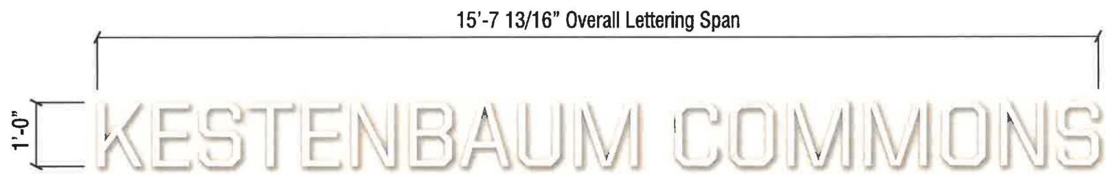
5 FRONT VIEW / SIGN ST-04 / BRUSHED STAINLESS STEEL REVERSE-PAN CHANNEL LETTERS (NON-ILLUMINATED) SCALE: 1/2" = 1'-0" QUANTITY: ONE (1) SET
