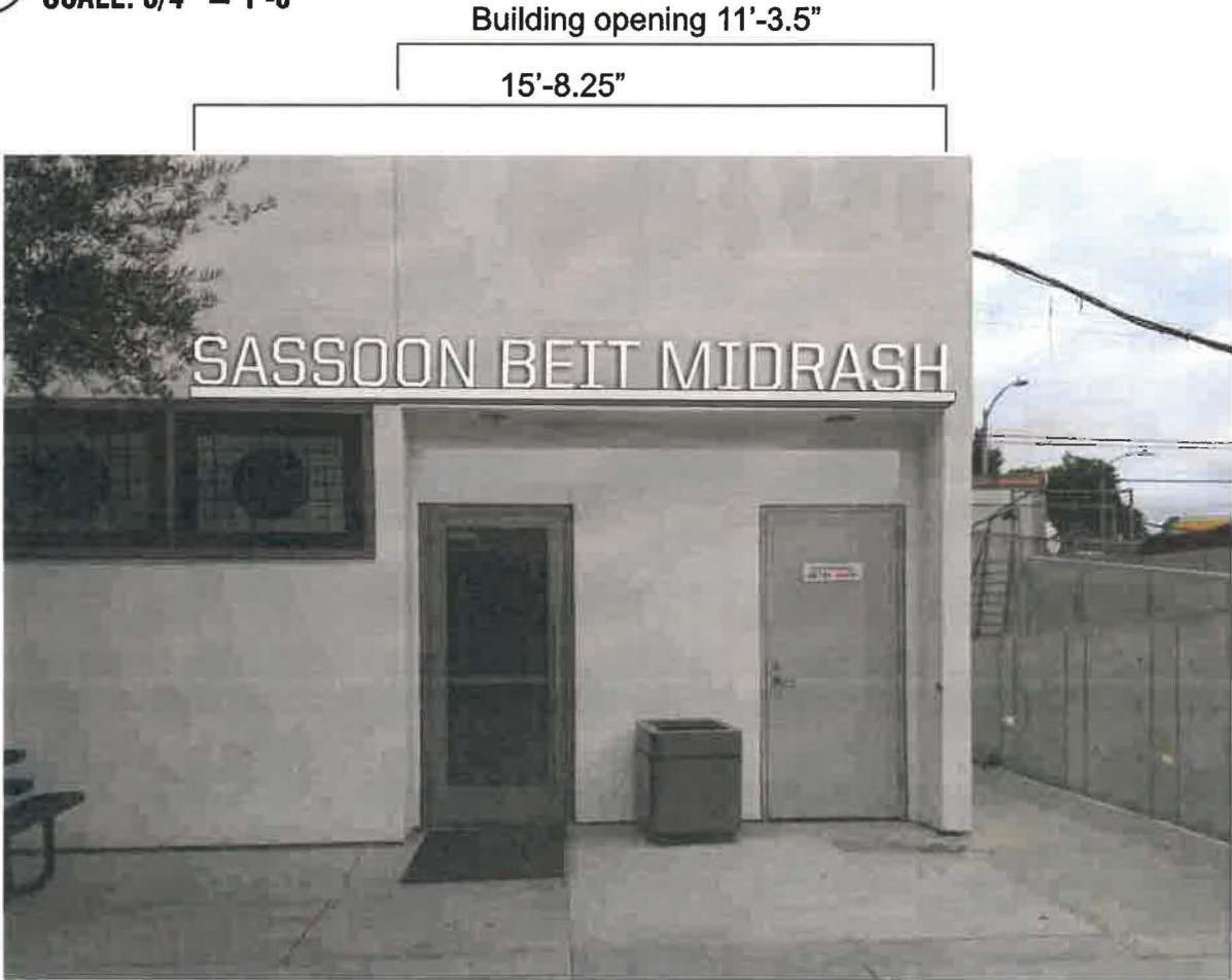
1 FRONT VIEW / SIGN ST-22 / STAINLESS STEEL REVERSE-PAN CHANNEL LETTERS ON A SHELF (NON-ILLUMINATED) SCALE: 3/4" = 1'-0"
