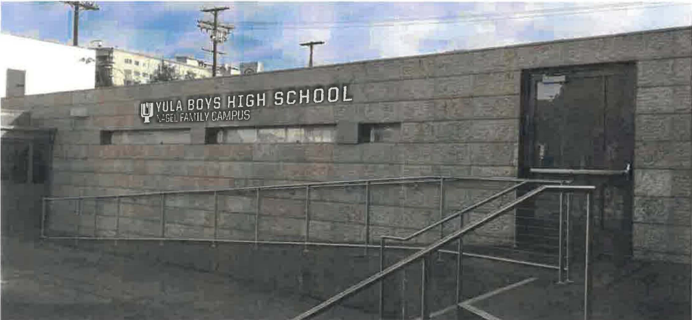
2 PHOTO WITH PROPOSED SIGN SUPER IMPOSED . / SIGN ID: ST-02b /FRONT VIEW / PROPORTIONS AND SCALE APPROXIMATE. STAINLESS STEEL REVERSE-PAN CHANNEL LOGO & LETTERS / (NON-ILLUMINATED) SCALE: NTS
