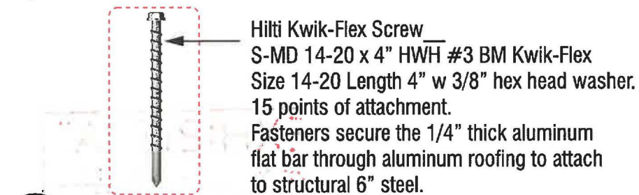
3 ATTACHMENT HARDWARE OF PROPOSED SIGN / SIGN ST-07 /
