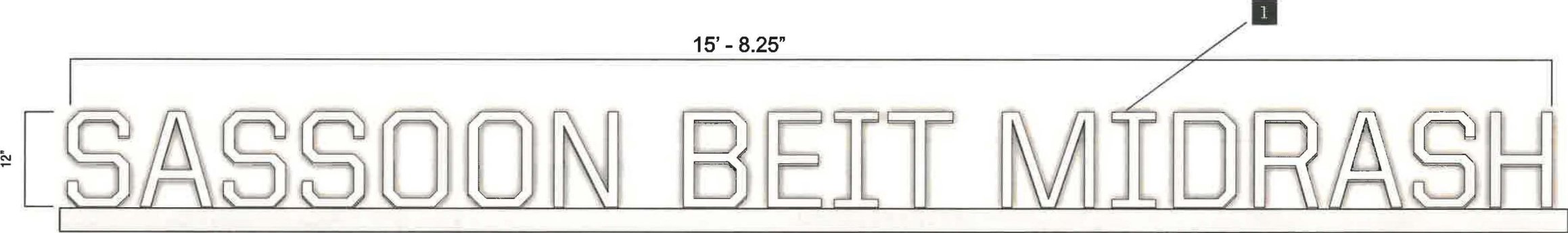
1 FRONT VIEW / SIGN ST-22 / STAINLESS STEEL REVERSE-PAN CHANNEL LETTERS ON A SHELF (NON-ILLUMINATED) SCALE: 3/4" = 1'-0"
